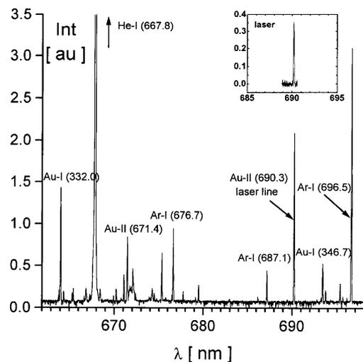
Fig. 4. Spectrum of the spontaneous emission of the laser tube with the identification of the most important transitions (wavelength given in nm units). Some of the lines originate from the second-order spectrum of the spectrograph. The inset shows the spectrum recorded while the laser was operating
