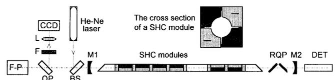
**Fig. 1.** The experimental setup and the cross section of a SHC module. M1, M2 – resonator mirrors, RQP – contra-rotating quartz plates, BS – beam-splitter, QP – quartz plate, F-P – Fabry-Pérot interferometer, F – filter, L – lens
