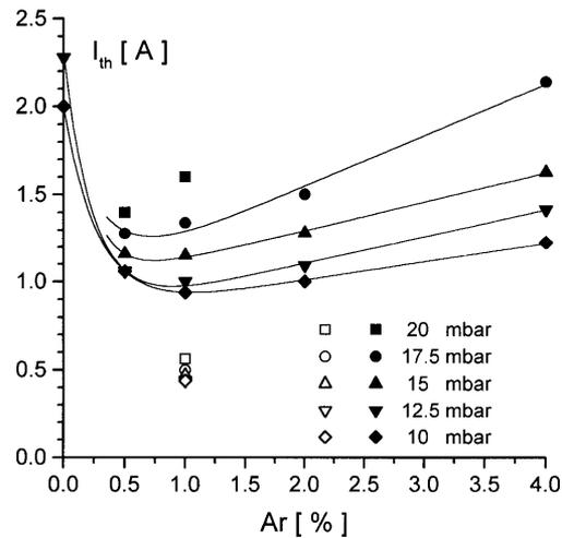
Fig. 3. Threshold current as a function of argon concentration. Solid symbols belong to results obtained with mirrors having curvature of 2 m while six SHC modules formed the active region. Open symbols: 3-m mirrors and five modules
