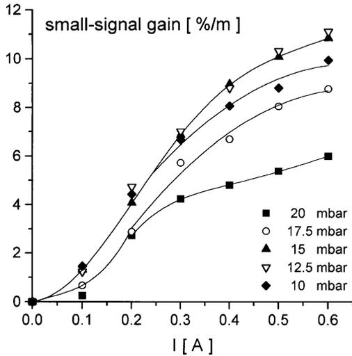
**Fig. 8.** Small-signal gain as a function of discharge current on a single module at different pressures
