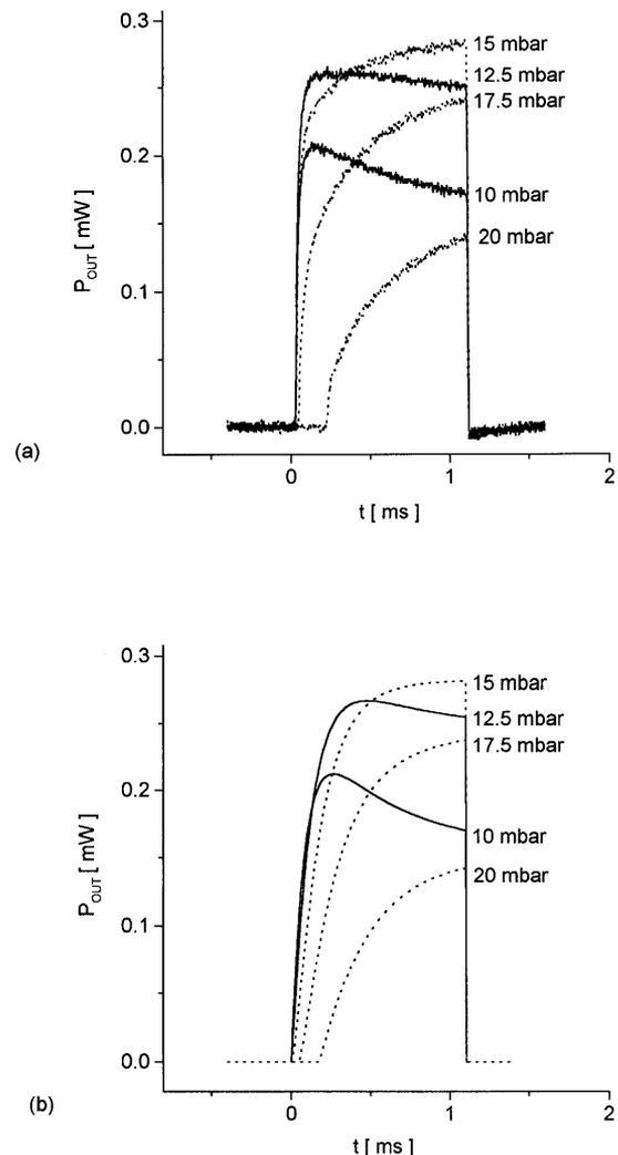
**Fig. 6a,b.** Time dependence of the laser output power obtained at different buffer gas pressures for  $I = 2$  A (five modules were used). **a** Measured data. **b** Results of the model
