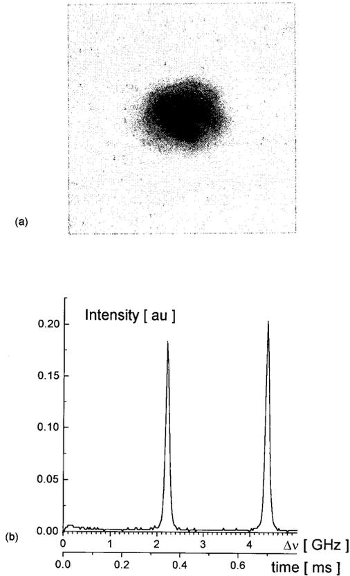
**Fig. 5.** **a** Intensity distribution in the cross section of the beam. **b** Frequency spectrum of the laser obtained with 3-m mirrors. ( $p = 17.5$  mbar,  $I = 3$  A)
