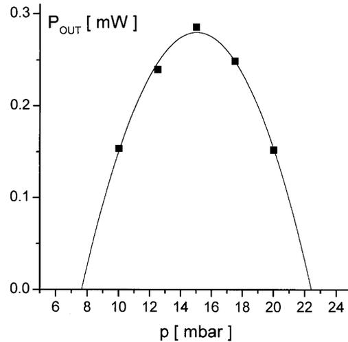
Fig. 7. Output power as a function of pressure obtained by the extrapolation of the measured curves (Fig. 6a) towards longer times
