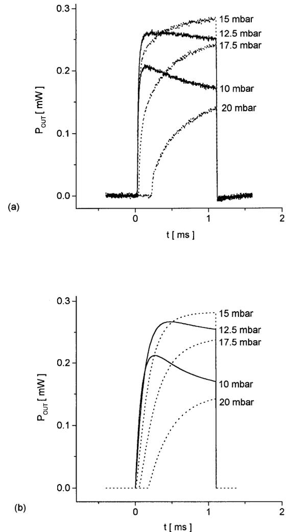
**Fig. 6a,b.** Time dependence of the laser output power obtained at different buffer gas pressures for  $I = 2$  A (five modules were used). **a** Measured data. **b** Results of the model
