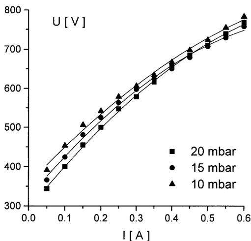
Fig. 2. Discharge voltage as a function of the current measured for one 5.6-cm-long SHC module with 1% of Ar in the He buffer gas
